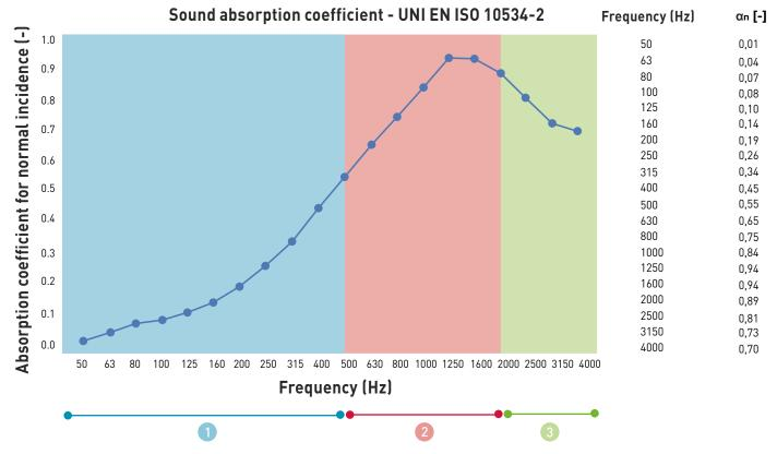
The sound absorption coefficient for normal incidence was calculated in Kundt's tube prepared according to the standard **UNI EN ISO 10534-2**, test executed by Materiacustica, a spin-off company of the University of Ferrara.
